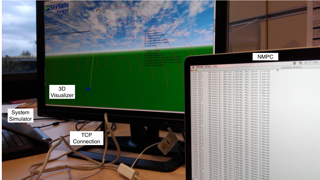
FIGURE 8.2: Experimental setup to test the NMPC using a TCP connection with the official Skysails simulator.
